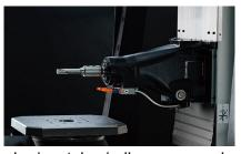
The horizontal spindle ensures a large machining area and enables the machining of large parts
