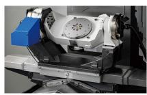
Equipped with a large tilting rotary table for machining large parts and multiple surfaces
