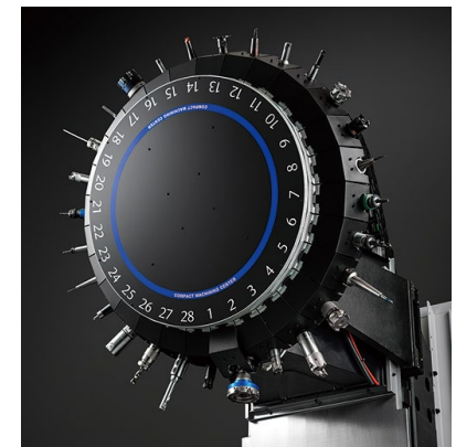
Equipped with a 28-tool magazine
