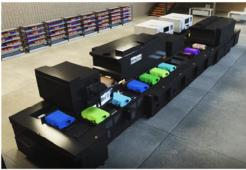
Image of the Digitalline automated garment printer line
