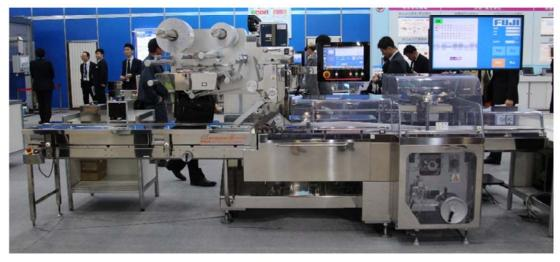
A FUJI MACHINERY high speed horizontal pillow packaging machine displayed at JAPAN PACK 2019 (the Vx 3-A is in the upper center)
