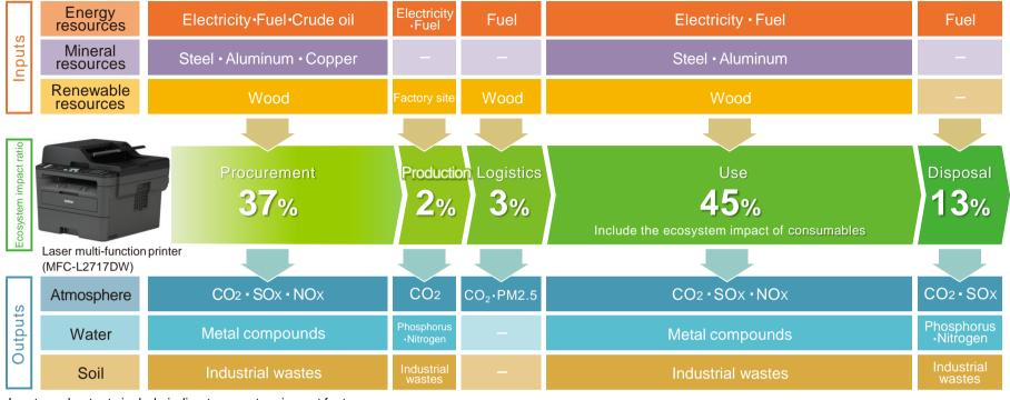
Inputs and outputs include indirect ecosystem impact factors.
